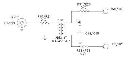
Figure 4. HMC960LP4E Evaluation Board Single-Ended Input Configuration
