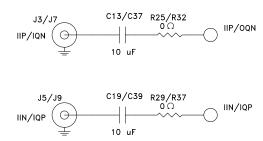
Figure 2. HMC960LP4E Evaluation Board Default Differential Input Configuration
